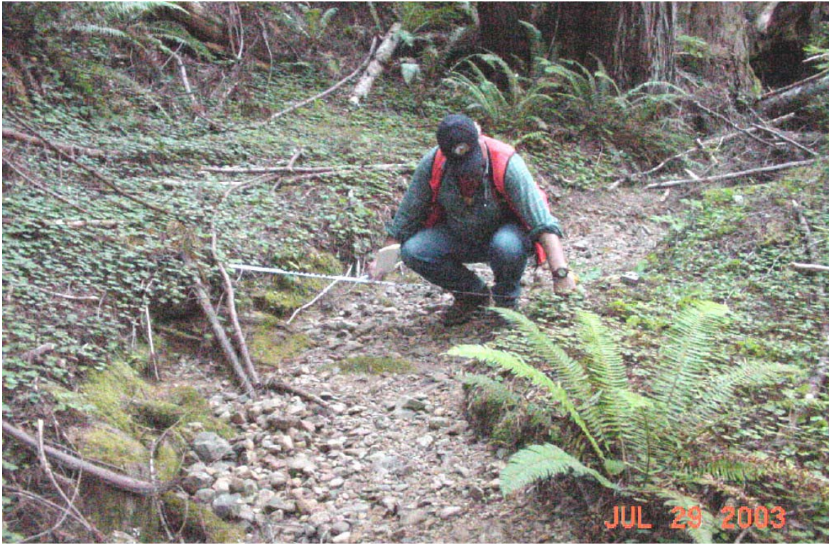
Figure 11. Clay Brandow, CDF Sacramento, measuring Caspar Creek sub-watershed HEN channel width for the 3 X bankfull stage calculation.
