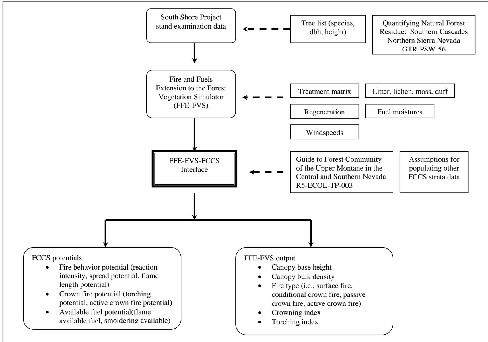
Fig. 1. FFE-FVS FCCS interface represents the flow of information between the FFE-FVS and FCCS.
