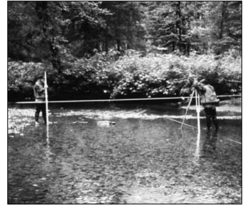
Measuring streambeds with professional surveying equipment increasing precision and the ability to detect changes in stream channel conditions.
