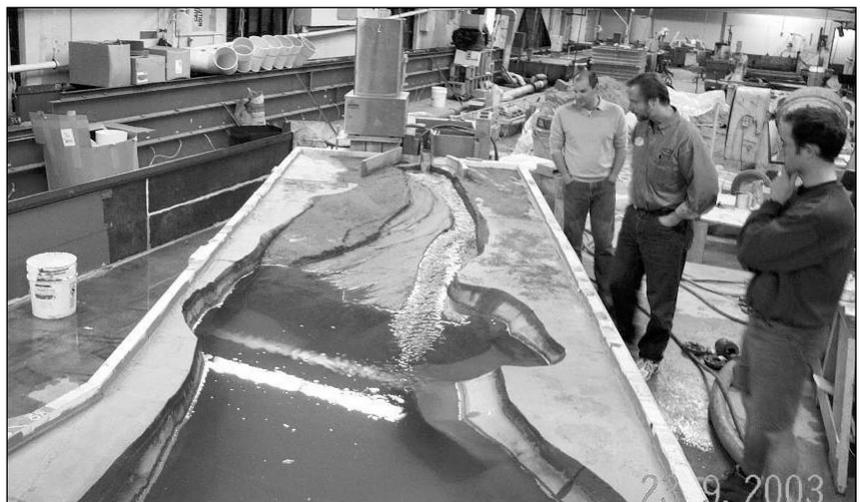
*A miniature version of the Glines Canyon Dam on the Elwha River in Olympic National Park, Washington, was constructed to model the release of sediment after the dam is removed in 2008. Photo by Gordon Grant.*
