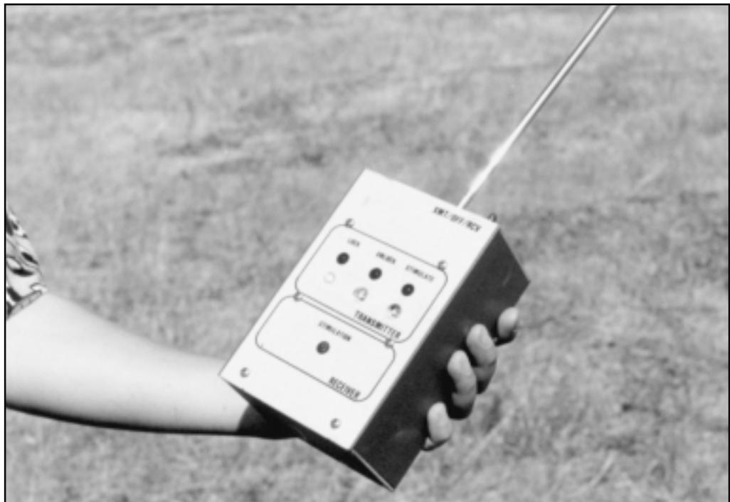
Figure 5—A hand-held unit enables us to lock, unlock, and stimulate eartags and to test the signal from the transmitter.
