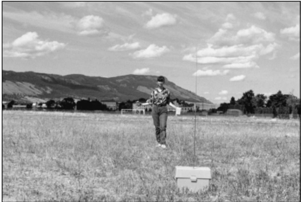
Figure 2—A transmitter housed in a plastic battery case emits a continuous coded signal. Signal distance is determined by approaching the transmitter with an electronic eartag and listening for the audio warning.
