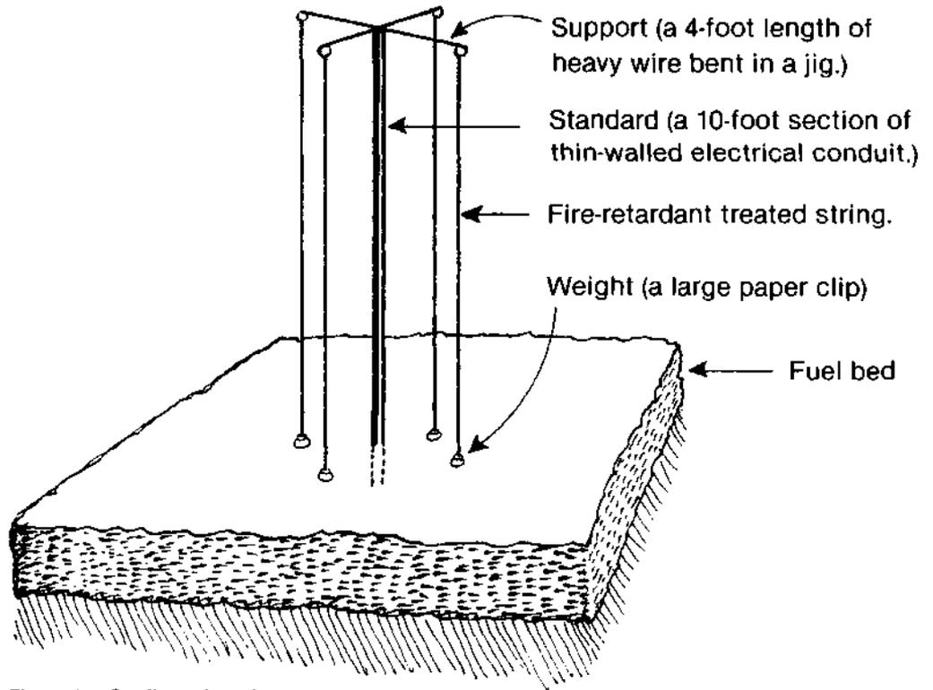
Figure 1.—Configuration of a flame-height sensor.
