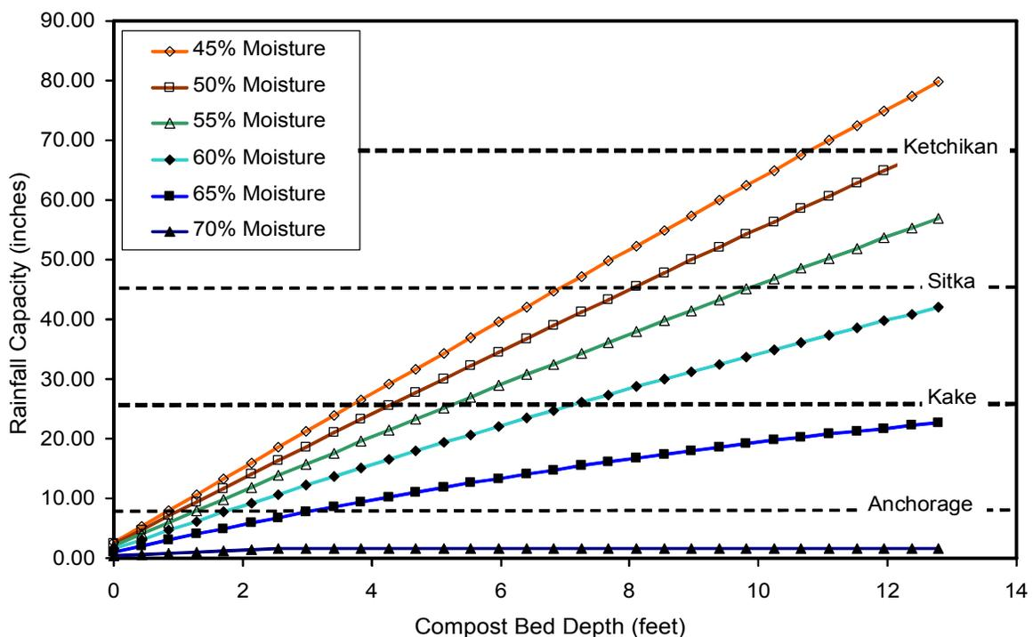
Figure 3--Cumulative rainfall absorption capacity for different depths of a compost bed, calculated for six moisture levels. The top of the pile (zero depth) is to the left.
