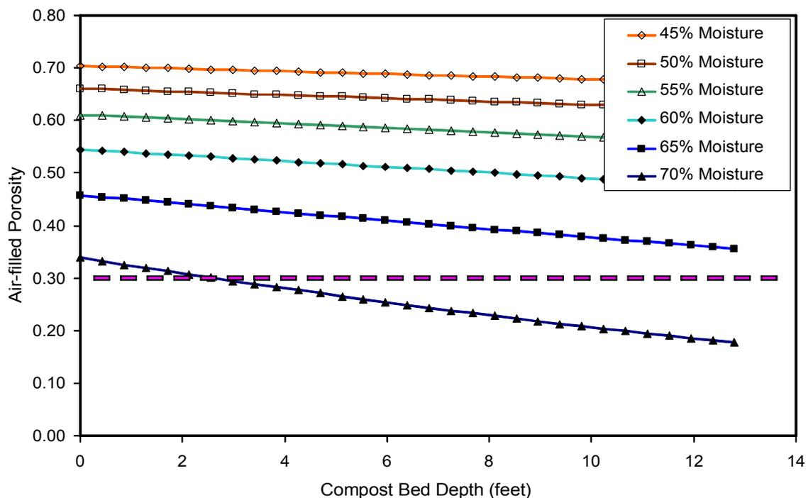
Figure 2--Air-filled porosity as a function of overburden compaction at different depths in a compost bed. The top of the pile (zero depth) is to the left.
