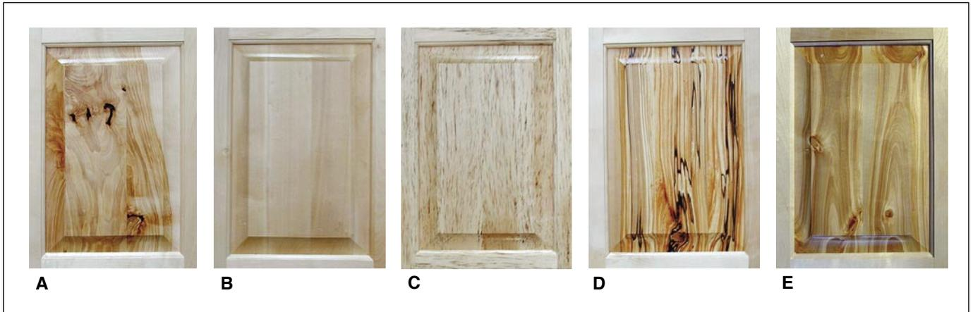
Figure 2—Selected birch cabinet doors used in consumer preferences study: (A) high level of character marking, (B) clear (defect-free), (C) ray fleck, (D) spalted, (E) grain variation.
