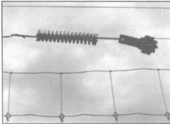
Figure 7—Typical in-line strainer.
