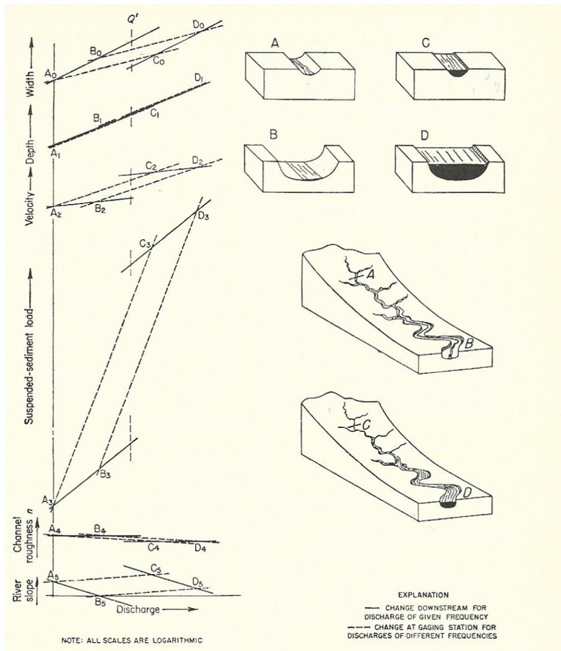
**Fig. 1.** Generalized hydraulic geometry relationships from Leopold et al. (1964) showing general trends for width, depth, velocity, suspended sediment, channel roughness, and slope. Note how trend lines convey continuity over the measured scales of discharge.
