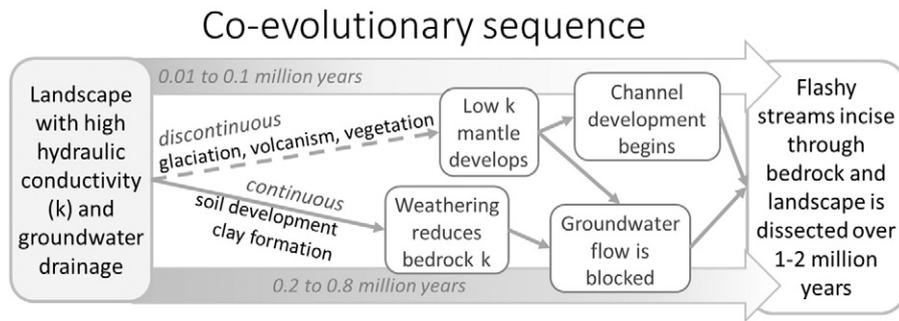
**Fig. 4.** Proposed trajectory for development of drainage density in the Oregon Cascades, after Jefferson (2006). Note that both continuous and discontinuous processes are actors in this scenario. While the continuous processes may take hundreds or thousands of years to play out, discontinuous processes acting over a much shorter timescales can jump start or accelerate the evolutionary sequence.
