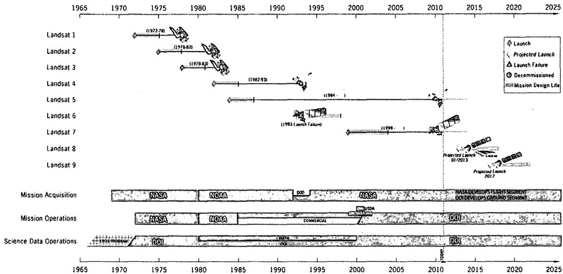
Fig. 1. Graphical illustration of Landsat program from EROS program inception in 1965 through present situation to anticipated launch of LDCM and beyond. Shown are launch dates, engineering design life objectives, and actual mission life spans. Also presented are science data, mission acquisition, and operations responsibilities.
