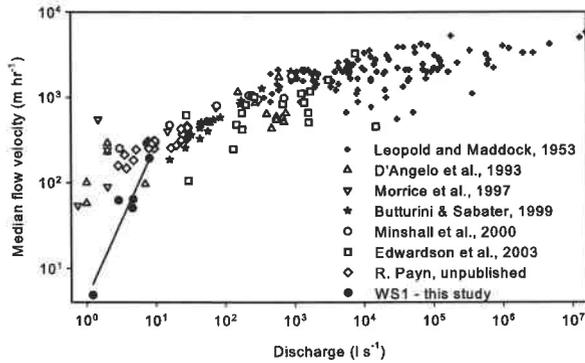
**Figure 1.** Discharge-velocity relations from a wide range of stream sizes and channel morphologies from gauging stations in a number of river basins and median flow velocities from stream tracer tests. Data and regression relation is also shown for flow velocities measured from tracer tests in the WS01 watershed ( $u = 4.57Q^{1.78}$ ;  $r^2 = 0.93$ ).
