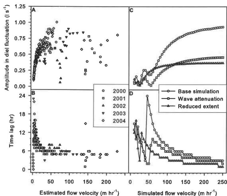
**Figure 3.** (a) The amplitude of diel fluctuations in stream discharge and (b) the change in time lag between the time of daily maximum  $ET_0$  and the time of minimum stream discharge over the period of baseflow recession. Model simulations showing (c) the relation between stream flow velocity and the change in the amplitude of diel fluctuations in discharge, and (d) the change in the time lag between maximum ET demand and daily minimum stream flow.
