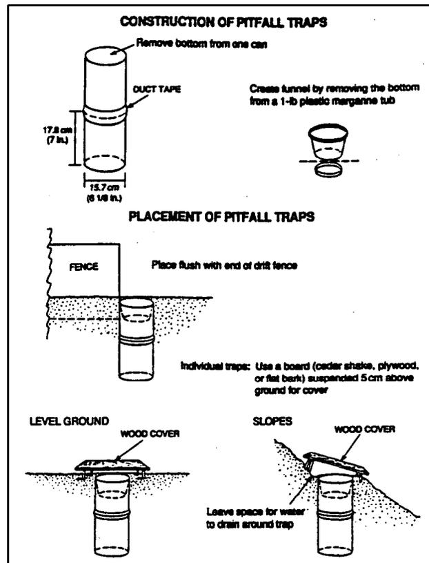
Figure 4-Construction and placement of a pitfall trap.
