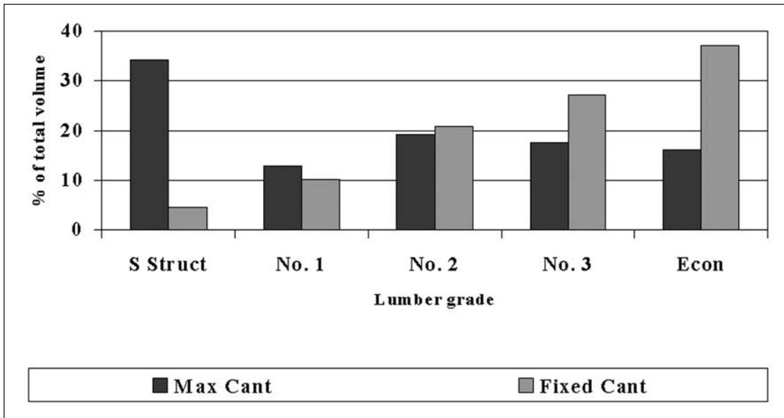
Figure 3—Effect sawing pattern on lumber grade from plantation-grown Douglas-fir logs greater than 20 inches in diameter when they are sawn to a fixed 4 and 6 inch cant widths or to the maximum cant that would fit into the log up to 12 inches (data from McConchhie et al. 1995, Kimberley et al. 1995).
