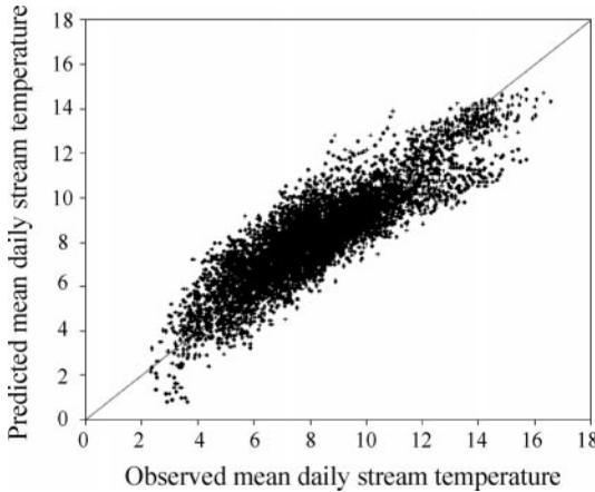
FIGURE 2.—Comparison between observed and predicted mean daily stream temperatures (°C) from a multiple-regression model using air temperature, elevation, and channel gradient. A 1:1 line is included for reference.
