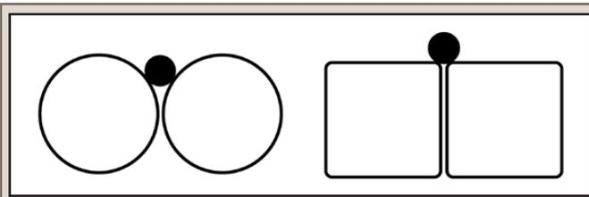
FIG. 1. Profile view of original (round PVC, left) and modified (square PVC, right) Salamander Stick that have equal diameter pipes. While Walston and Mullins (2005) use PVC pipes 2.54 cm in diameter (i.e., larger than our modified Salamander Stick), we depict both versions having equal diameter. Solid black dots represent salamanders of equal diameter, and illustrate their placement when pulled into the crevice.
