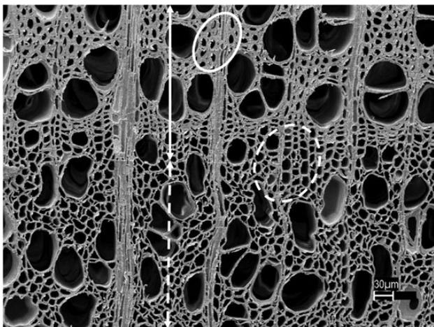
**Figure 4.** SEM micrograph showing the difference in fiber cell wall thickness between normal-colored portion of the ring (upper half with solid white circle and white arrow) and dark portion of the ring (center and lower half with dashed white circle and dashed white arrow).
