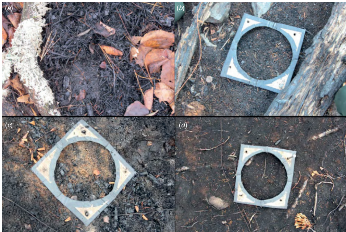
Fig. 2. Example of soil fire burn severity classes: (a) class 1, >85% forest floor remaining; (b) class 2, 40–85% forest floor remaining; (c) class 3, 1–40% forest floor remaining; and (d) class 4, 0% forest floor remaining.
