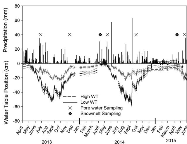
**Figure 1.** Mean water table positions (in cm below the peat surface) in the low and high WT treatment mesocosms and precipitation (in mm) over the course of this study from 2013 to 2015. Water table manipulations were conducted in the summer months, while water table levels were left to stabilize during the winter months. Dashed lines around the low and high WT treatment mean water table positions represent the 95% confidence interval. Pore water and snowmelt sampling events are denoted.
