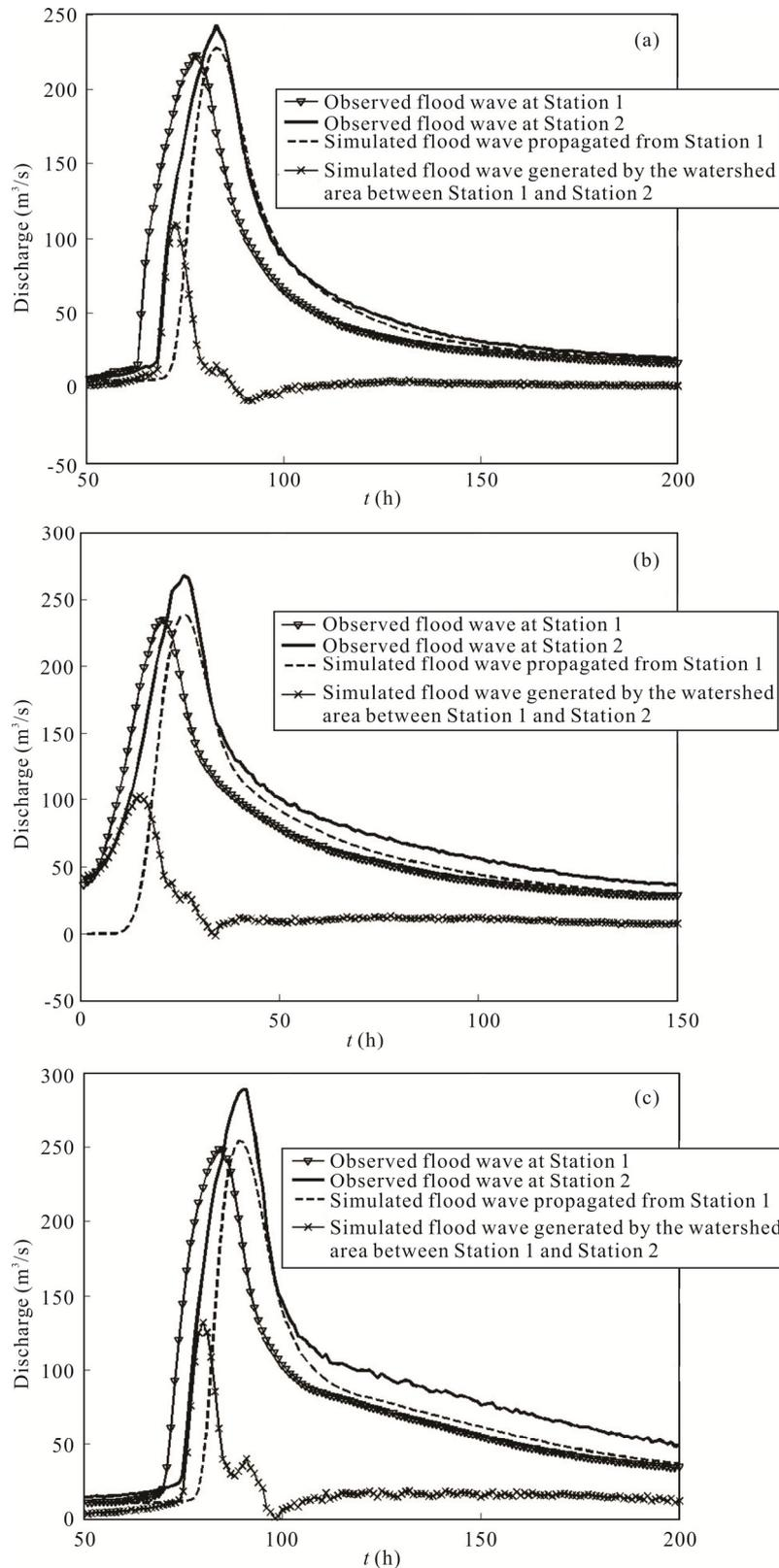
**Figure 3.** Observed and simulated flood waves. (a) flood wave on January 29, 2013 to February 4, 2013, of which the river bed roughness was calibrated; (b) flood wave on April 27, 2013 to May 3, 2013; (c) flood wave on November 15, 2009 to November 21, 2009.
