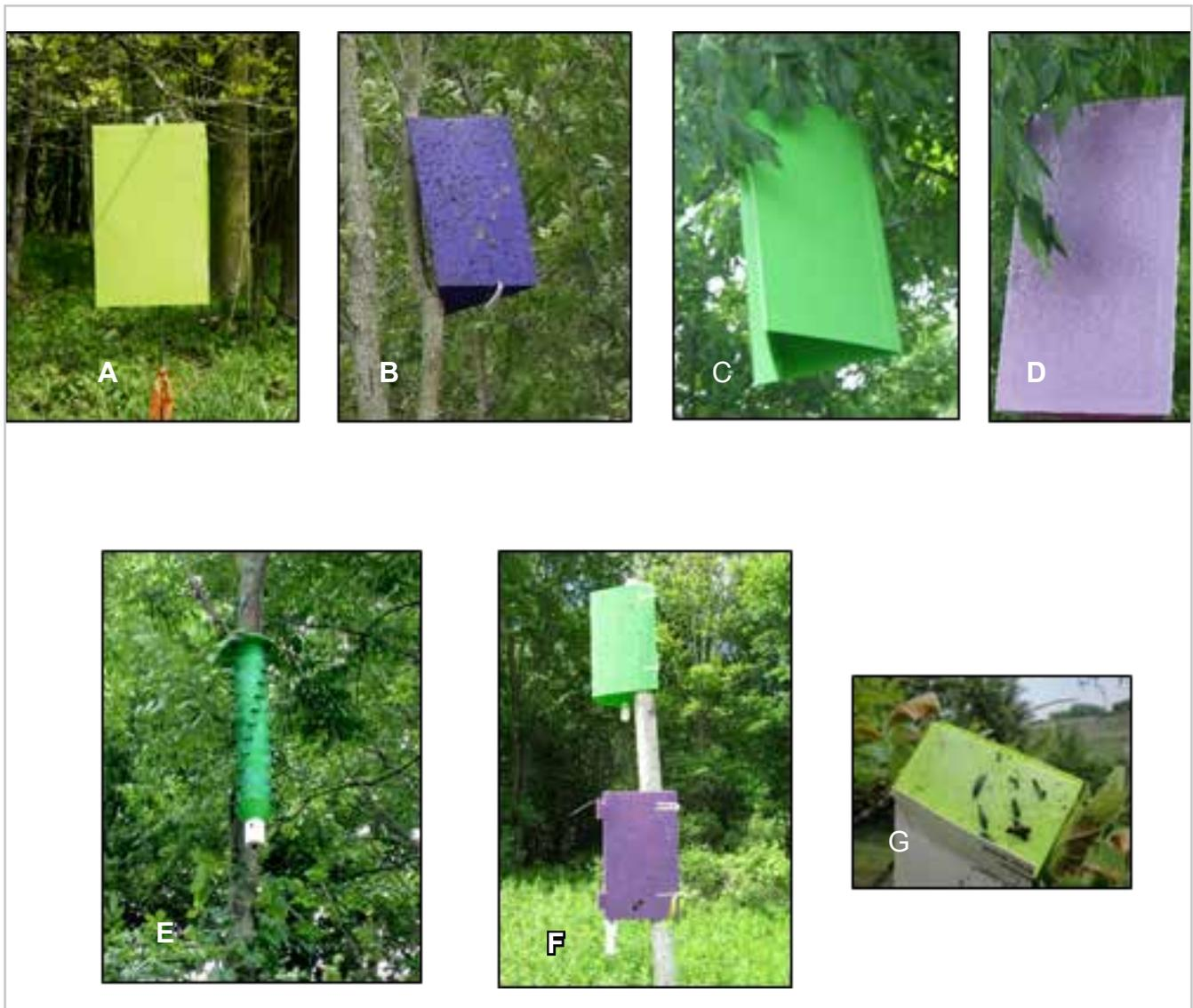
Figure 1. Traps used for capturing EAB. A. Light green prism trap; B. Dark purple prism trap; C. Dark “Sabic” green prism trap; D. Light “Sabic” purple prism trap; E. Dark “Sabic” green multiple funnel trap; F. Double-decker trap; G. Light green branch trap
