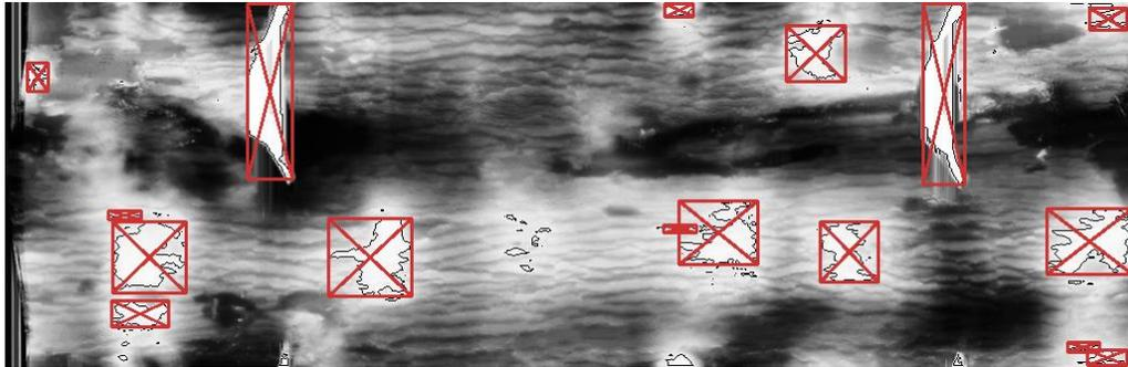
Figure 4—Residual image of log 31C with contour levels and defects identified using the parallel algorithm.
