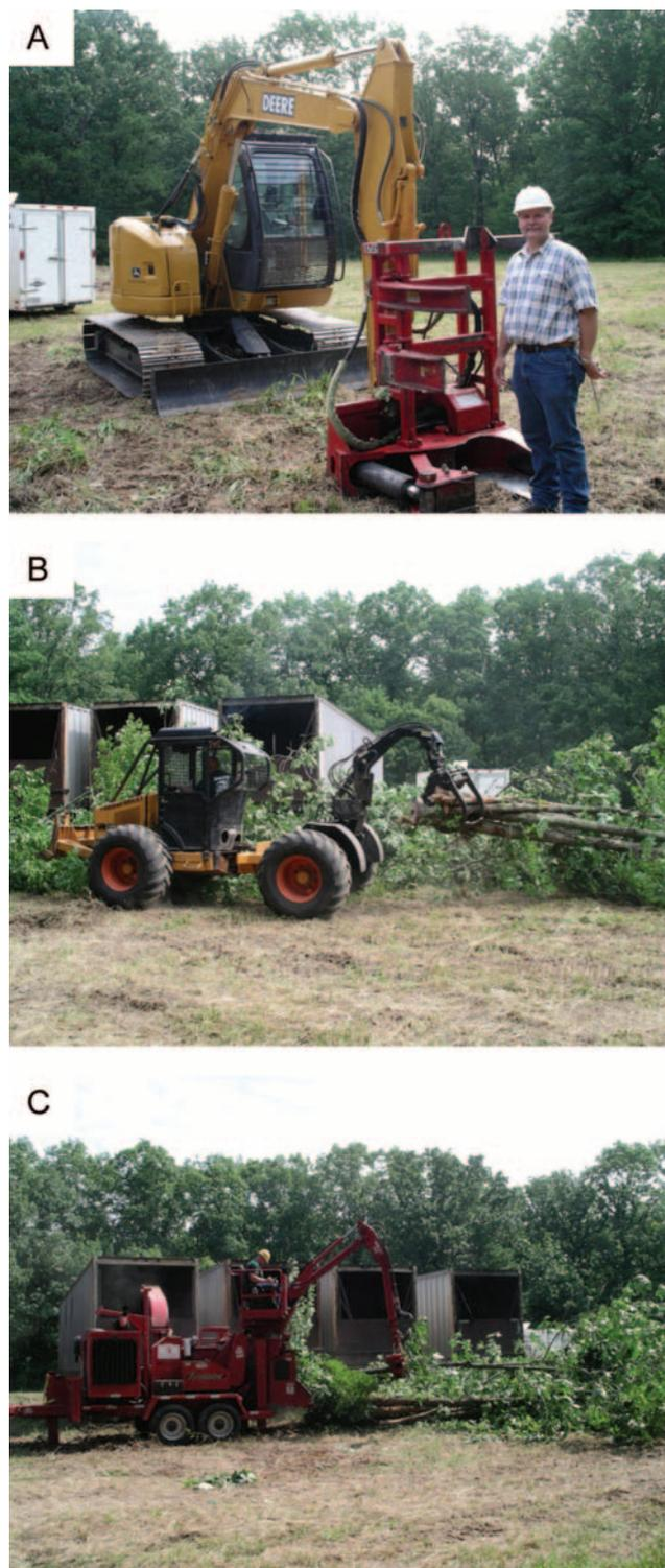
**Figure 1.** Felling was completed by a small excavator (John Deere 75C) with a Fecon shear head (A). Felled trees were placed in bundles that were transported to the landing using a 50 hp hydrostatic Turbo Forest skidder with a swing-arm grapple (B). Bundles taken to the landing were chipped using a 325 hp Morbark Typhoon chipper equipped with a small loader (C).
