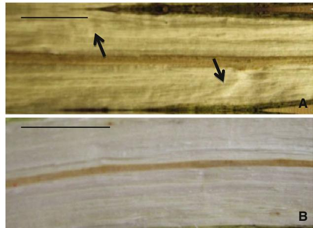
**Fig. 2** Radial surfaces of xylem after a split test from **a** 11-month-old Curly Poplar, showing undulations (arrows), and **b** 11-month-old clone 4877, with straight grain and a smooth surface. Scale bar = 1 cm
