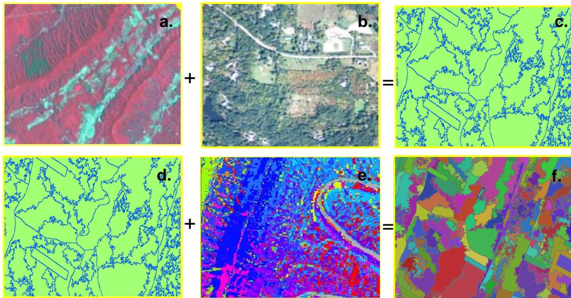
**Figure 2. Methodology overview. 30-m Landsat imagery (a) was combined with 1-m NAIP imagery (b) using the resolution merge procedure to create a 5-m multispectral input image for segmentation. ECognition software was used to segment this image (c). The polygons from image segmentation (d) were combined with a 30-m output from a WEKA-based image classification (e) to produce the final, classified stand map (f).**
