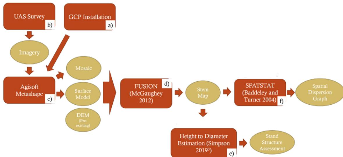
Figure 2.—UAS image processing and analysis workflow.
