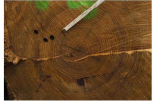
Figure 15.—Bore damage in the butt log of white oak. This log also exhibits slow and fast growth rate, ring shake, and very poor color.
