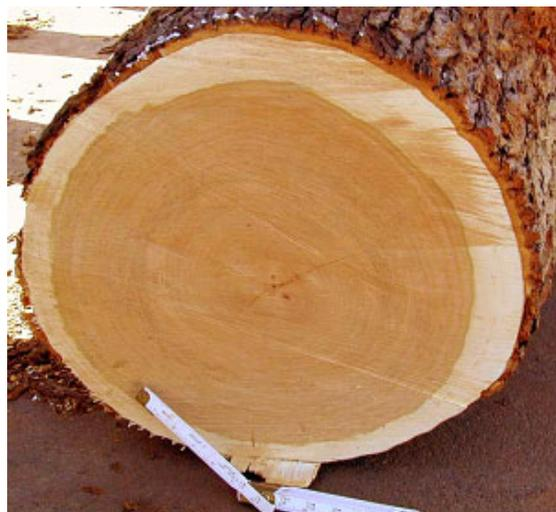
Figure 6.—Cherry log showing irregularity in the concentricity of the growth rings or “Tear Drop” which causes a dimple effect in the veneer sheet.
