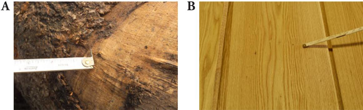
Figure 14A, B.—Pin knots in a white oak log (A) and in the veneer (B).
