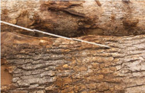
Figure 16.—Bulges at the base of some large white oak, also called “coke bottle effect” are not considered defects.
