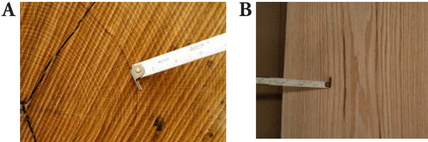
Figure 13A, B.—Mineral stain following a growth ring on the end of a white oak log (A) and appearance of mineral in white oak veneer (B).
