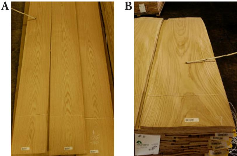
Figures 12A, B.—Note the unique light color and centered uniform cathedral of the white oak flitch (A) as compared to the coarse, irregular flitch (B).
