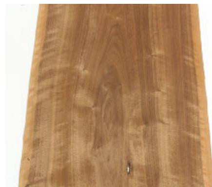
Figure 7.—Figure or flash in walnut veneer. Small amounts of figure as shown here are usually not desirable. A highly figured flitch, on the other hand, commands a premium price.
