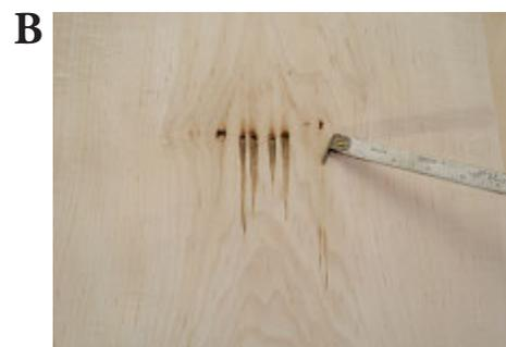
Figures 20A, B.—Bird peck on a hard maple tree (A) and resulting defect in the veneer (B).
