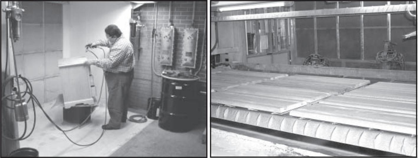
Figure 11.—Case-finishing (left) versus component flat-line finishing (right).
