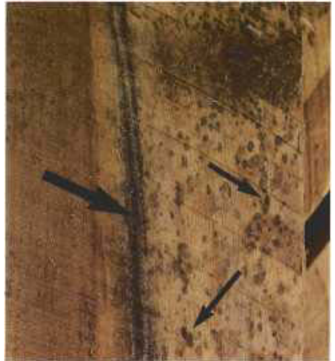
Figure 7.--As drying progresses, the dark stain columns fade to a light greyish tan (right side of board) and healthy tissues gradually darken (left side of board). Note the dark smudgy strip where C. virescens (large arrow) has grown out onto wood surface near the edge of the stain column, and the blotchy colonies of saprophytic mold fungi (small arrows) growing exclusively on the sapstreak diseased wood.
