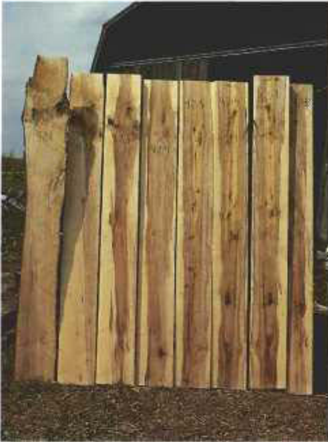
Figure 6.--Boards cut from the log of a sapstreak diseased tree. Note extensive columns of dark discoloration.
