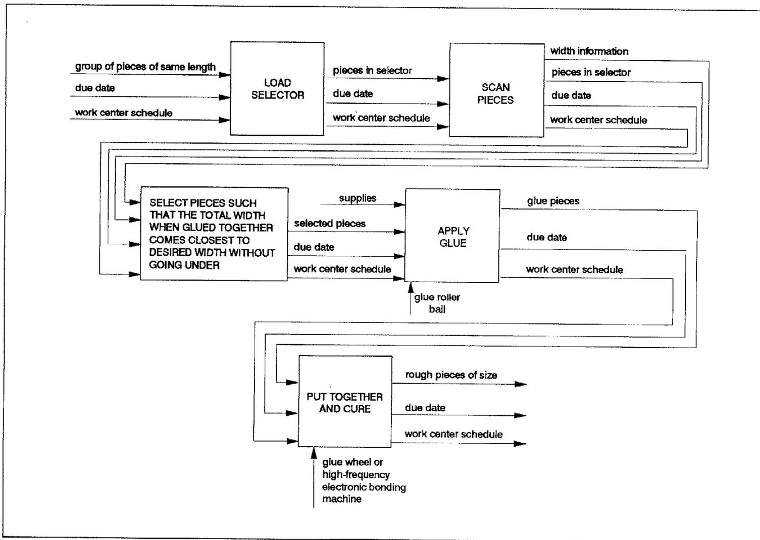
Figure 16.—1A35 Glue boards together.
