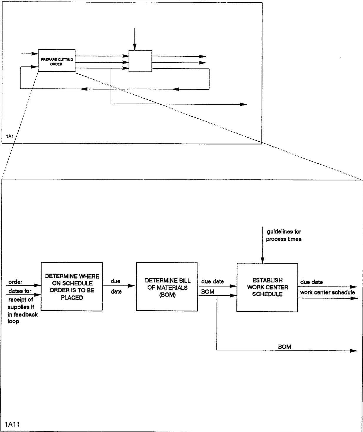
Figure 4. —Decomposition of prepare cutting order.
