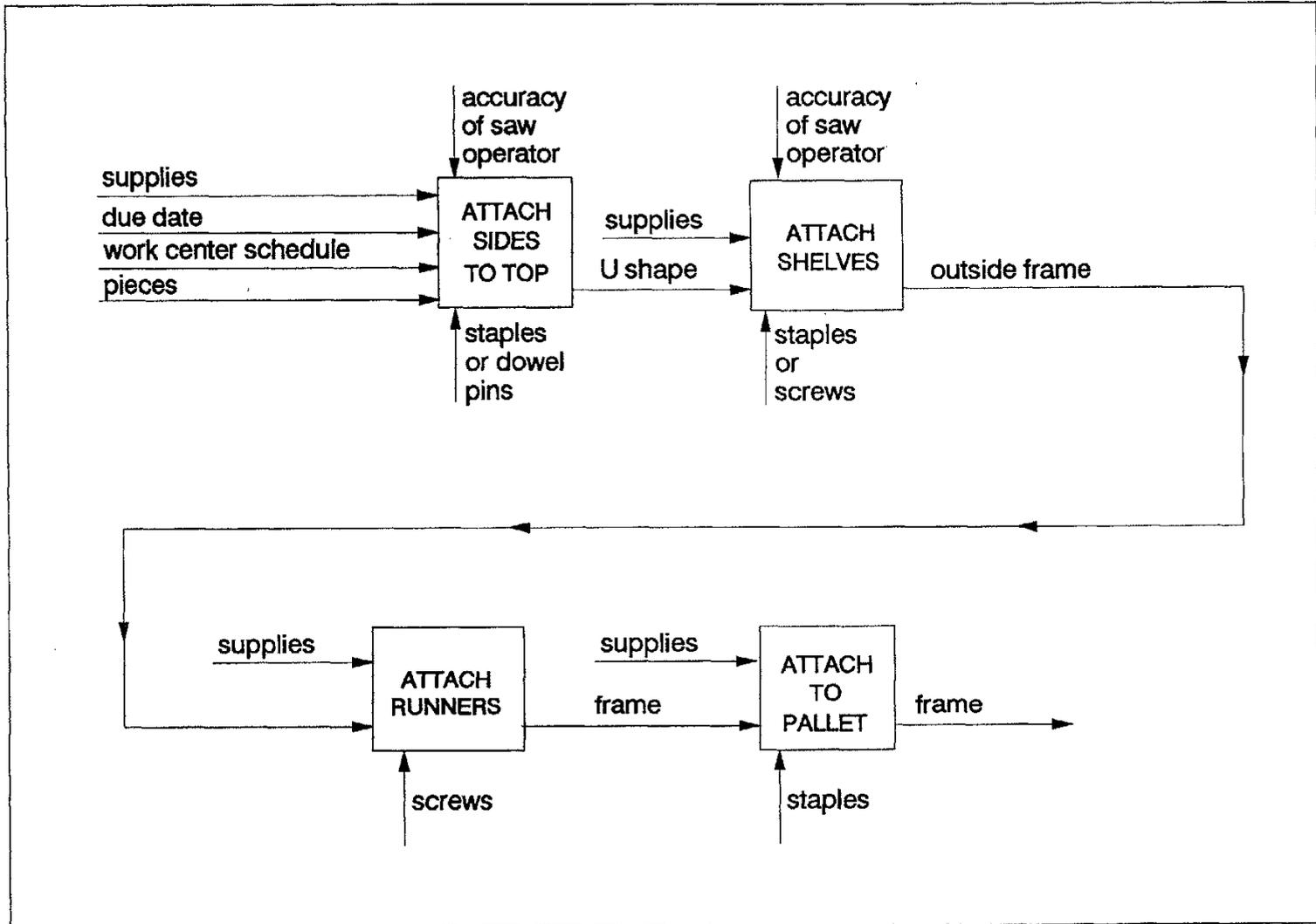
Figure 25. — 1A51 Assemble frame.
