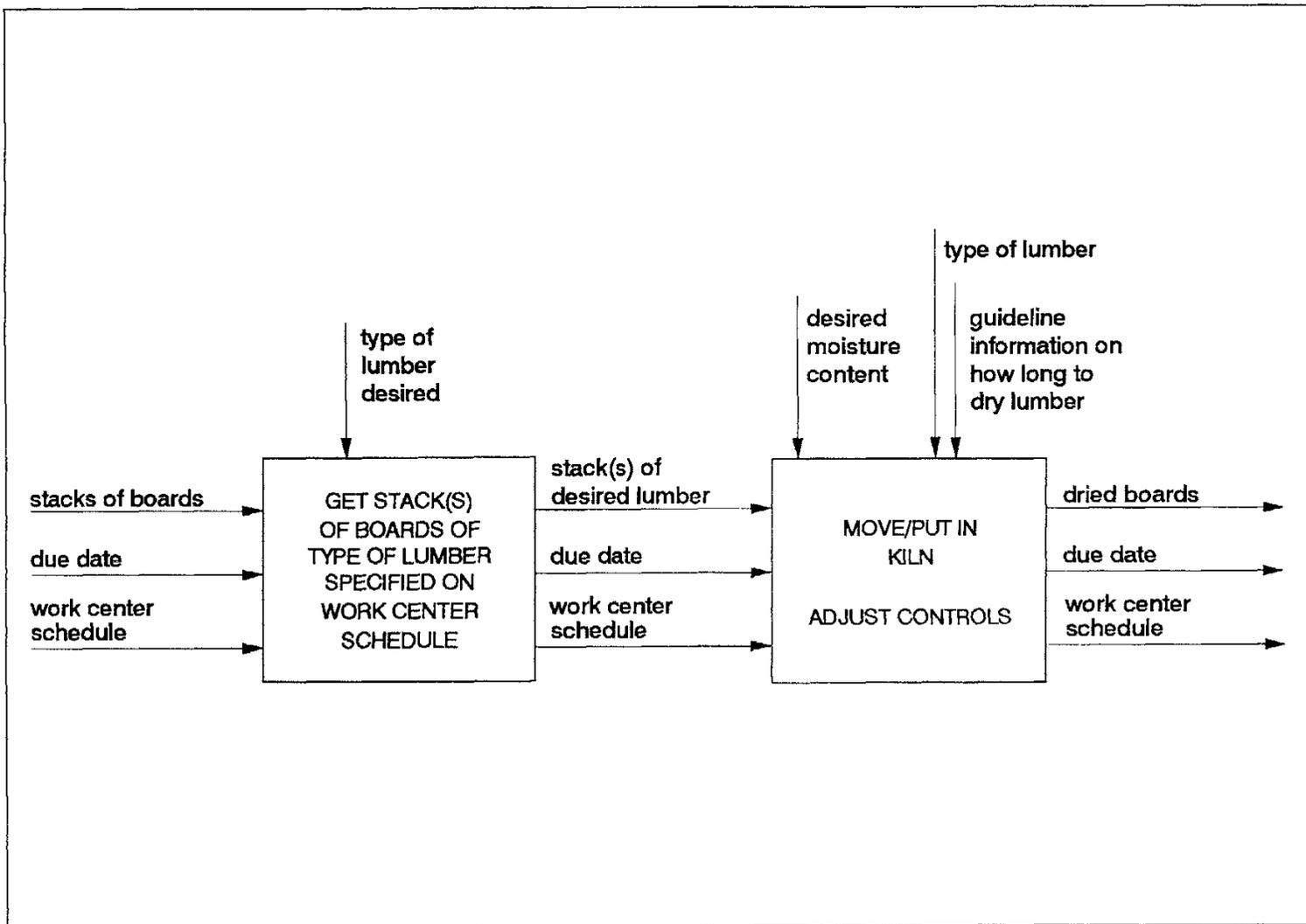
Figure 12.—1A22 Kiln dry boards.
