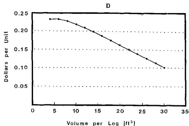
Figure 2.—Incremental effects of skidding variables on costs for Holder Tractor for following conditions (mean values): (a) slope yarding distance, 800 feet; (b) number of logs per turn, 3; (c) turn volume, 30 ft<sup>3</sup>; (d) volume per log, 10 ft<sup>3</sup>.
