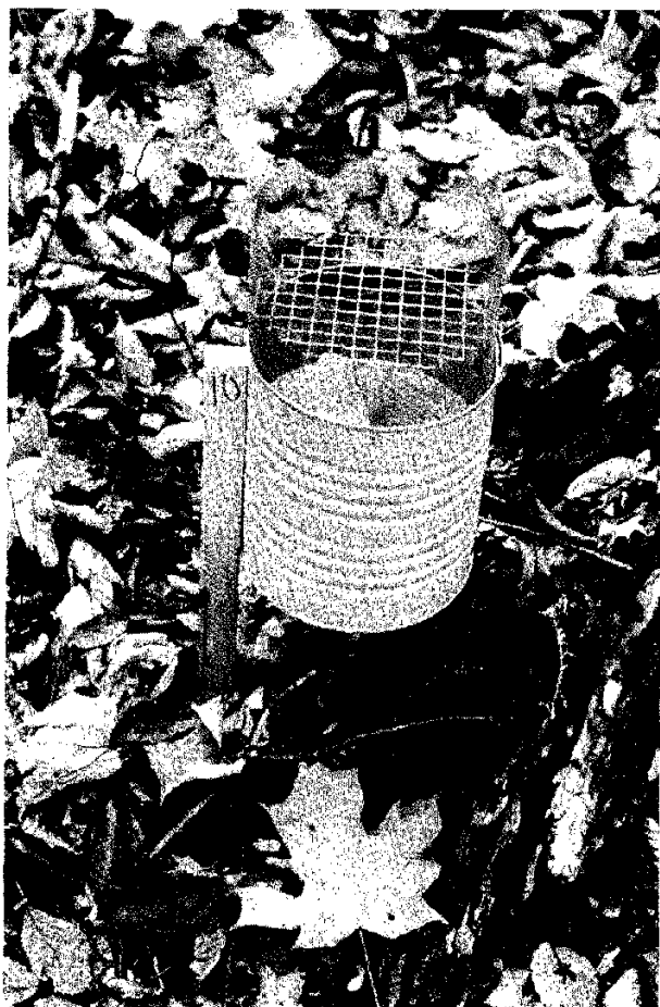
Figure 2.—Cylindrical seed trap as used during the growing season. The screen top reduced wind deflection during windy periods, increasing trap reliability.
