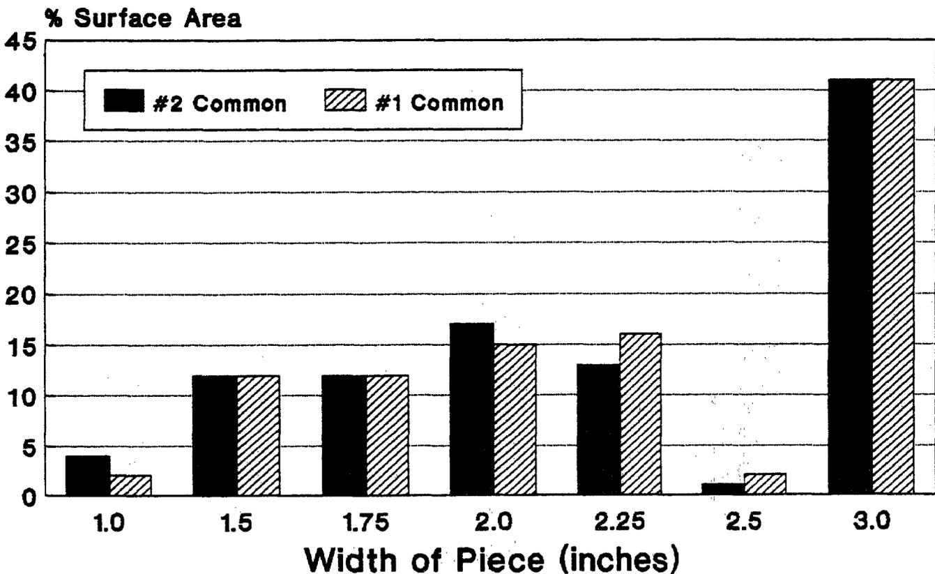
Figure 3.—Distribution of parts widths, crook removed, fixed-arbor saw spacings—widest first.
