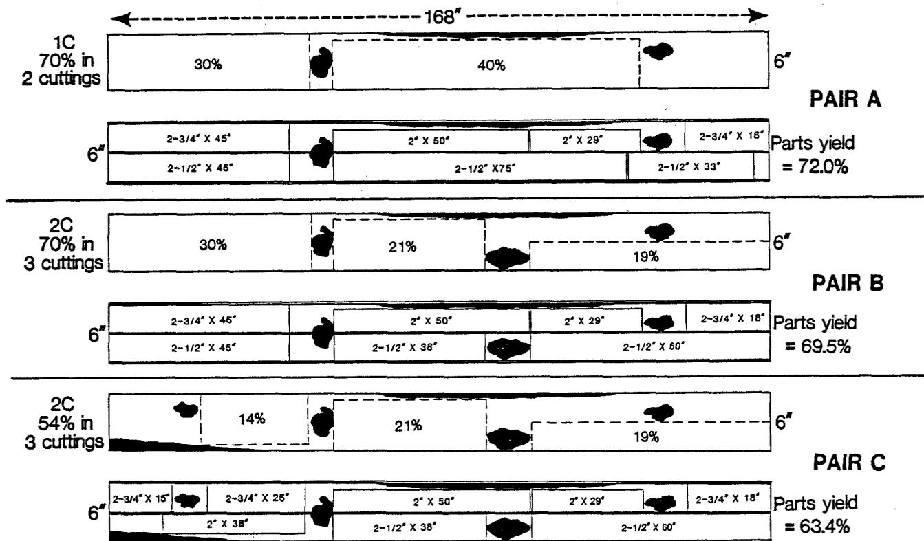
Figure 1.—Examples of the effects of decreasing grade on the yields from gang-ripping No. 1 and No. 2 Common lumber. Additional defects were added to Pair A to get the Pair B and Pair C boards. Drawing is approximately to scale.
