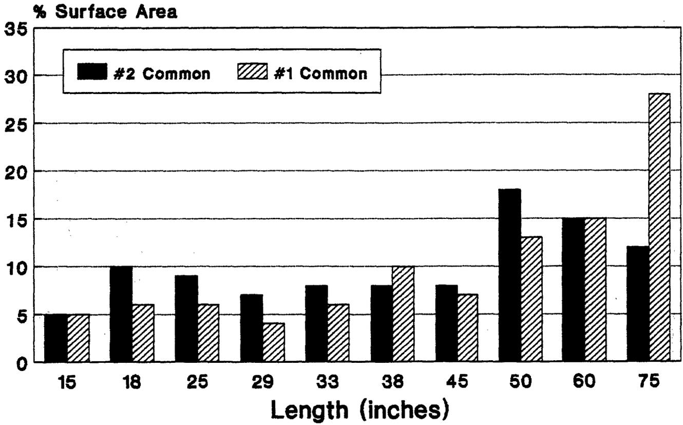
Figure 5.—Distribution of parts lengths, crook removed, fixed-arbor saw spacings—widest first.
