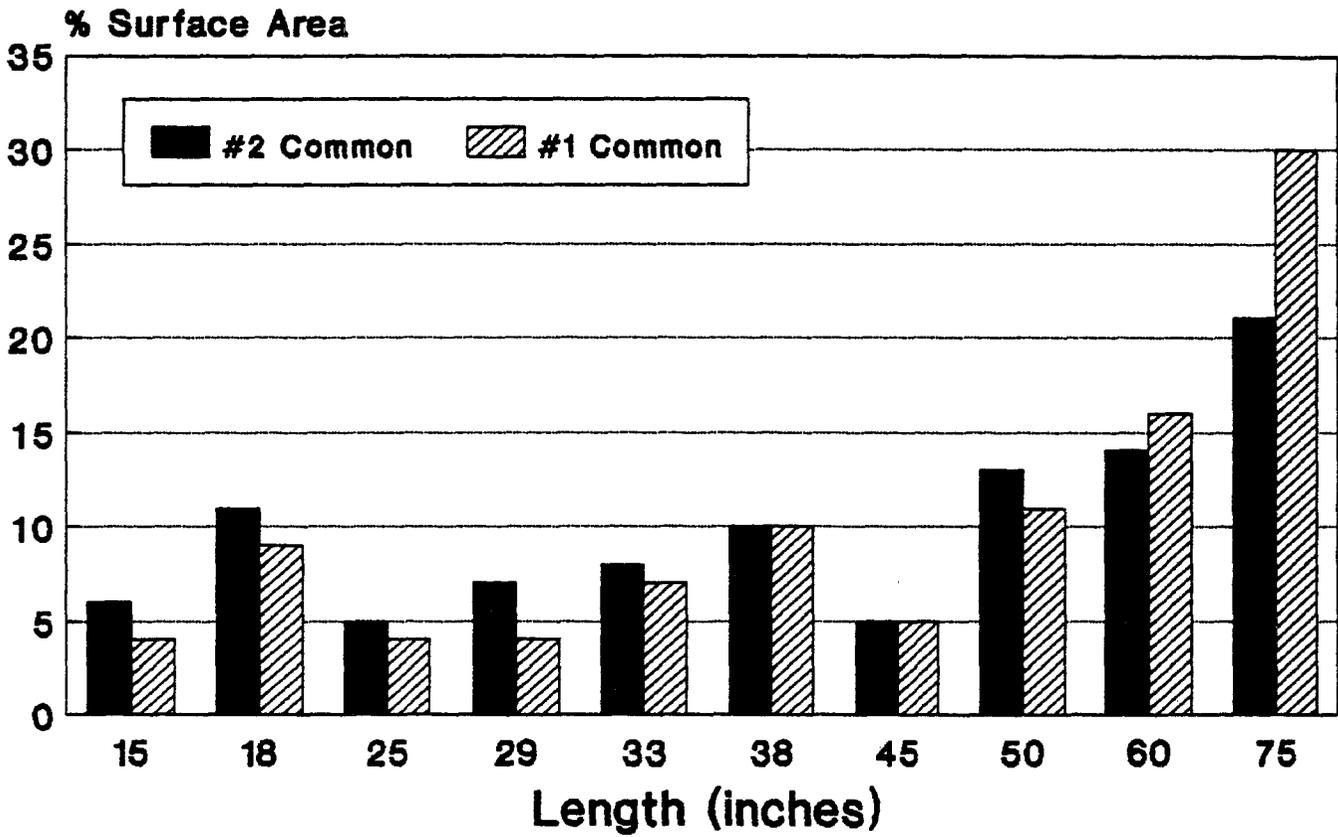
Figure 4.—Distribution of parts lengths, full-length boards with crook, fixed-arbor saw spacings—widest first.
