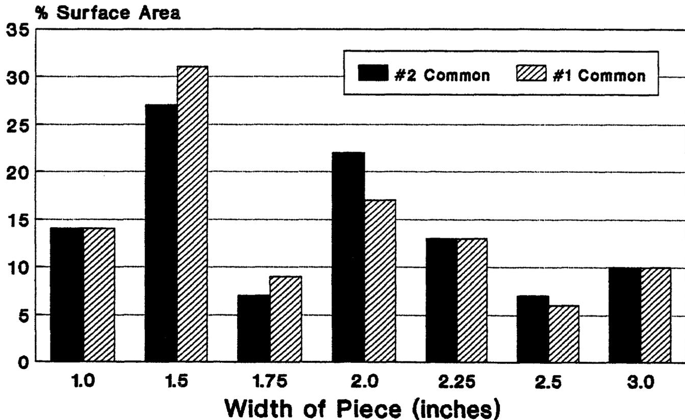
Figure 2.—Distribution of parts widths, full-length boards with crook, fixed-arbor saw spacings—widest first.
