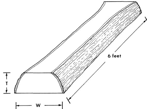
**Figure 2.—Measuring two-sided cants.**
