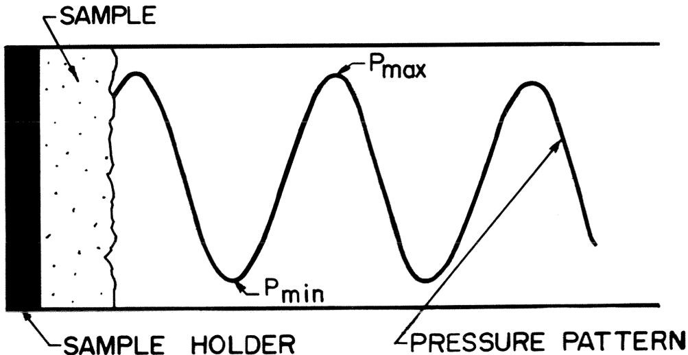
Figure 2.—A schematic diagram of the impedance tube apparatus.
