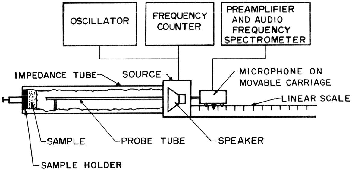
Figure 3.—The impedance tube, instruments, and several samples.
