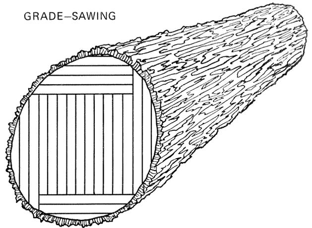
Figure 2.—Sawing patterns for live-sawing and grade-sawing.
