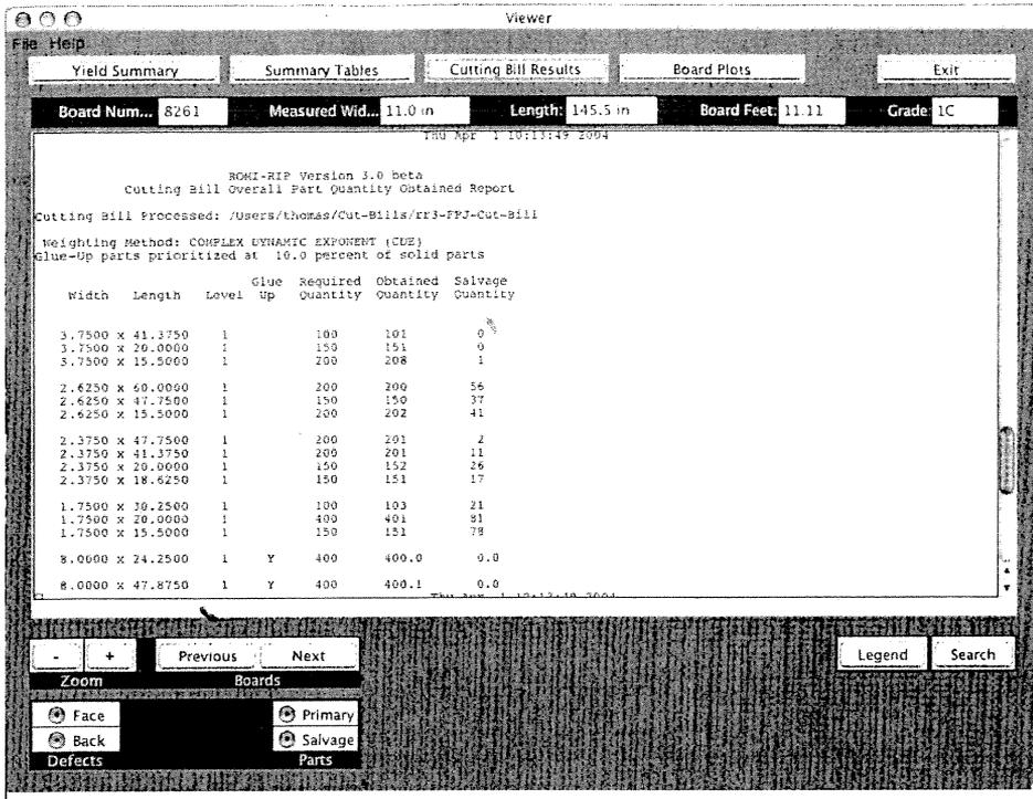
Figure 2. — Sample cutting bill report showing parts sizes, required quantity, and quantity obtained.
