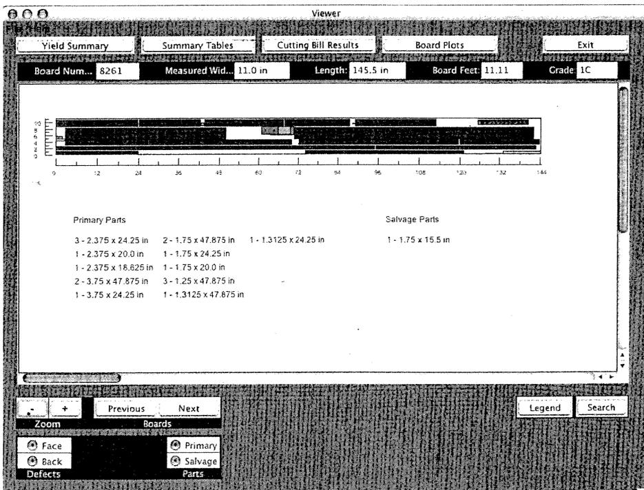
Figure 3. — Graphic showing cutting solution for a selected board.
