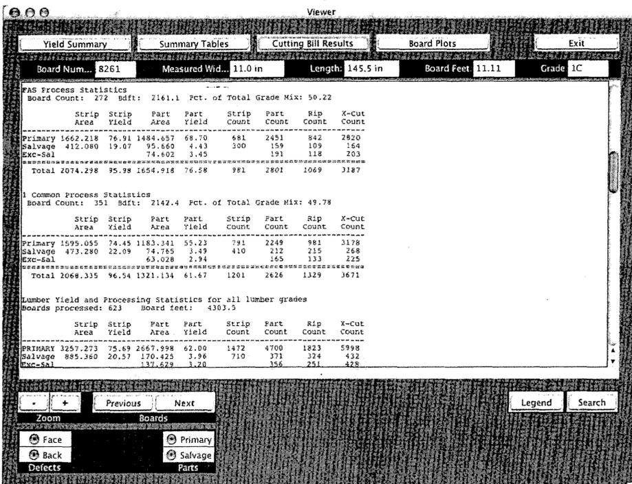
Figure 1. — Sample report showing yield and processing requirements by lumber grade.
