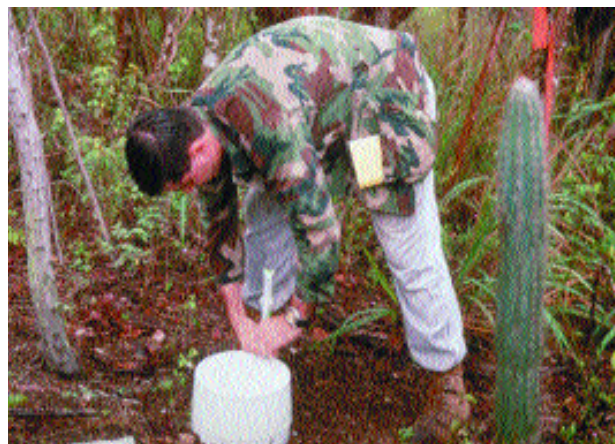
Sampling flux chamber headspace gas with a syringe in the drought deciduous forest of Guánica, Puerto Rico. The syringe samples are analyzed in the laboratory for \text{N}_2\text{O} and \text{CH}_4 concentrations by gas chromatography. Photo by H. Erickson
