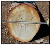
Scaling is the determination of the gross and net volume of logs. The primary purpose of scaling is to determine the volume by product or species to be charged at a predetermined rate.
