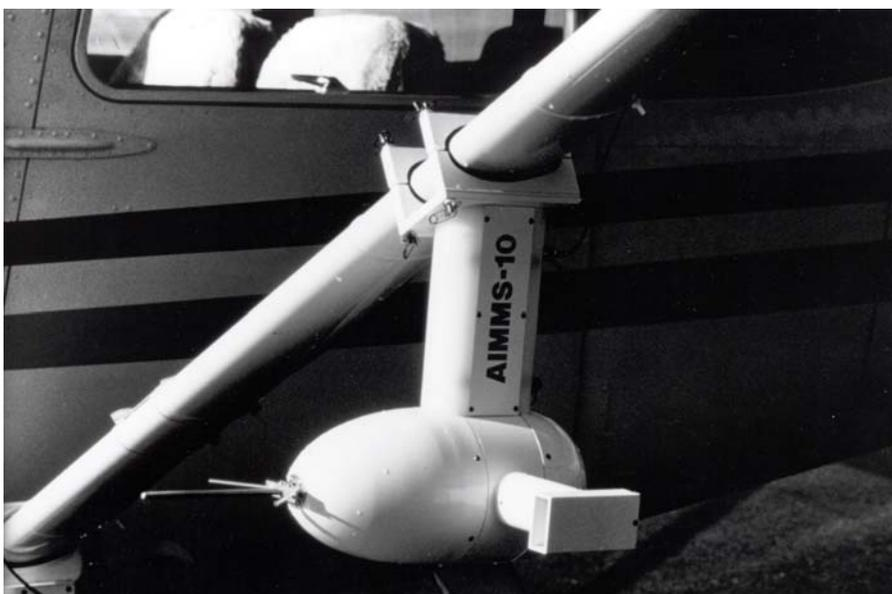
Figure 12—An aircraft-mounted meteorological sensor package was evaluated by the Center in 1997. Sensors transmitted the temperature, dew point, wind speed, and direction to a ground-based PC while simultaneously plotting the aircraft's position on an overlay map.
