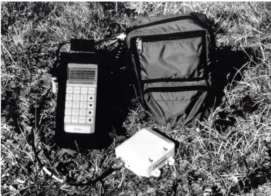
Figure 7—The GPS Support Program has evaluated data loggers capable of downloading data into Arc/Info and other GIS software.
