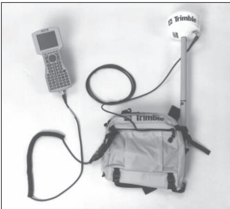
Figure 1—Trimble ProXRS GPS system: TDC1 data logger (left), GPS receiver (center), and integrated antenna (right). The antenna receives GPS signals and real-time DGPS corrections.
