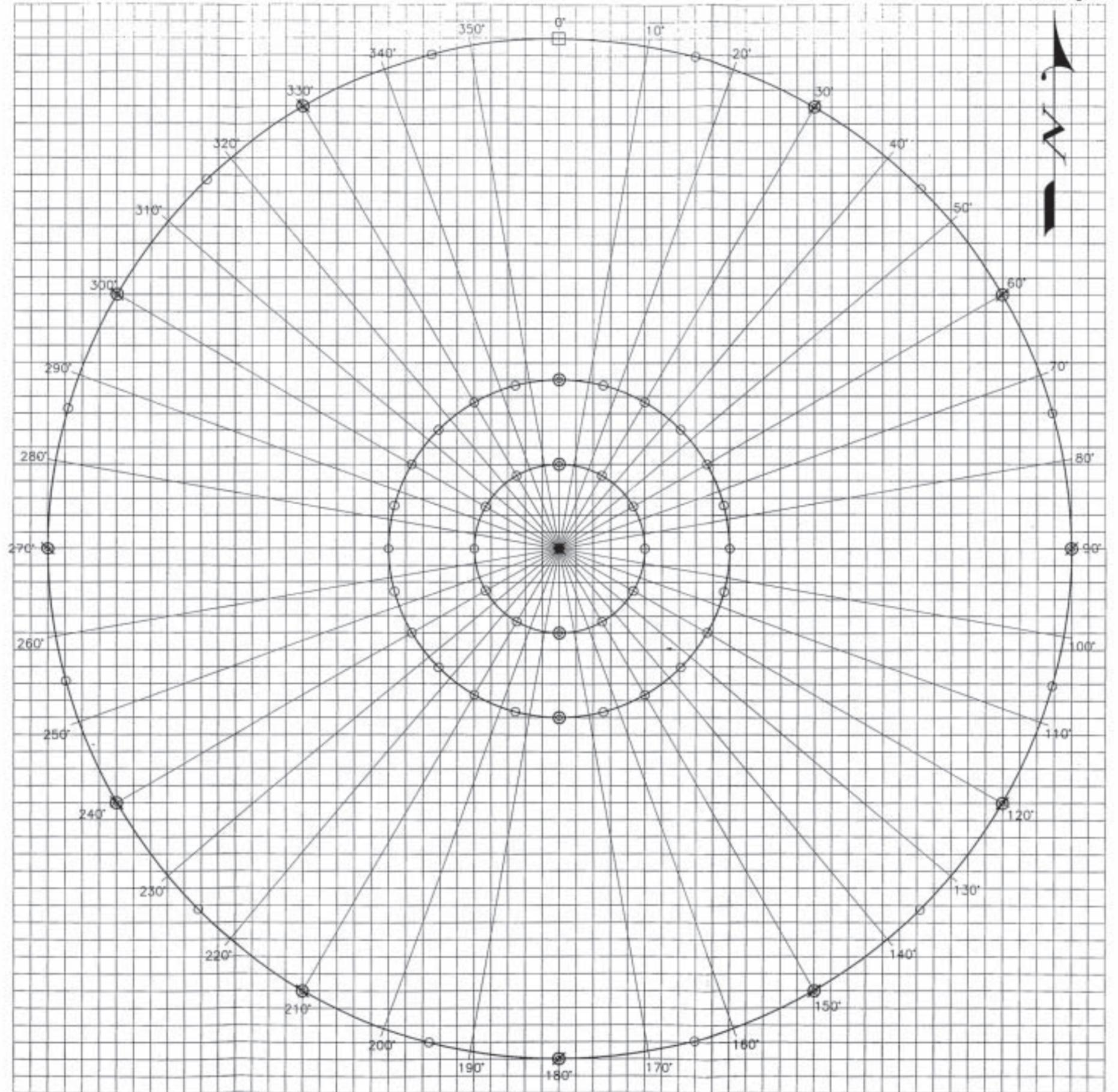
Figure 1—A set of three concentric circles are centered over the emission point and mark the sampler deployments.
