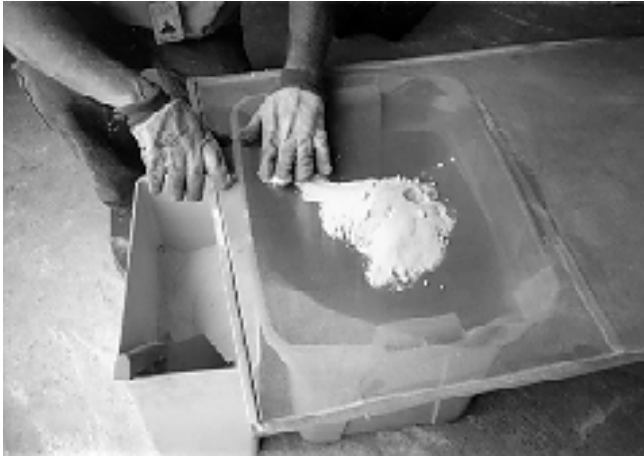
Figure 20a—Prepare Sporax by screening the material before placing it into the applicator reservoir.
