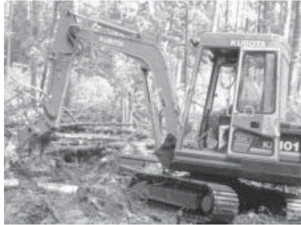
FERIC scarification rake mounted on a Kubota 101 excavator.
