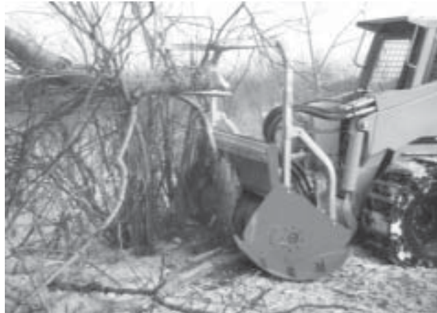
Seppi Midiforest mounted on a skid steer.
