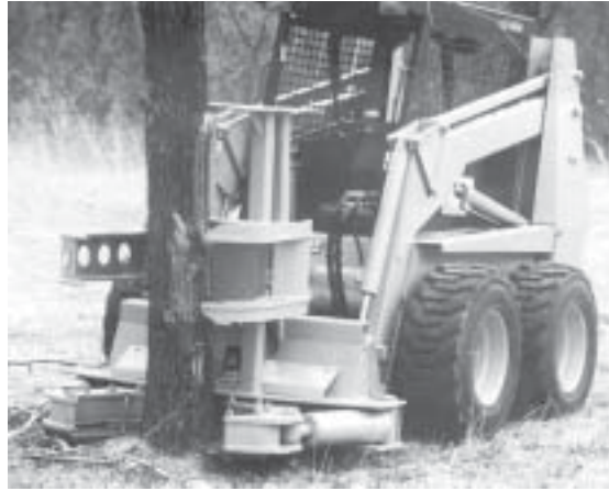
Dymax 14-inch forestry tree shear with accumulator, mounted on a skid steer.
