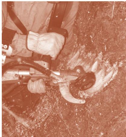
Figure 11—The Li'l Beaver has a semi-conical cutting head.
