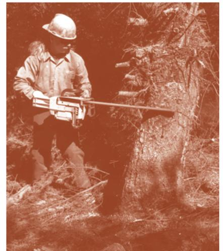
Figure 9—Chain saws are commonly used as girdling tools.
