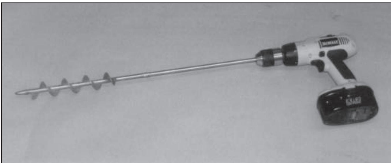
Figure 5—Battery-powered, 18-volt drill with auger.
