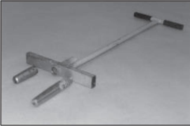
Figure 2—Hollow dibble with interchangeable heads. The heads are threaded into the base. Various-size heads can be used depending on container-stock size.
