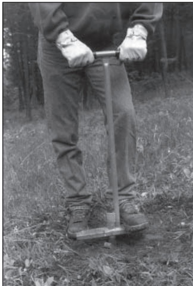
Figure 1—Planter using the hollow-dibble planting tool.
