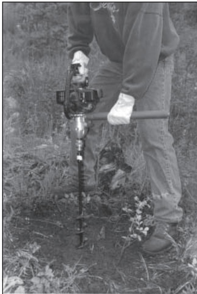
*Figure 4—Planter using Tanaka gas-powered drill with auger. The padded extension arm was added for leg protection and increased gripping area.*
