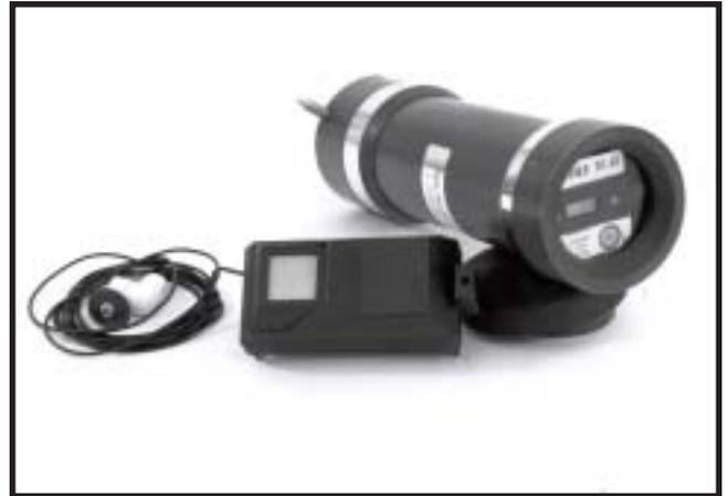
Figure 5—TR-41 trail traffic counter by Compu-Tech Systems.
