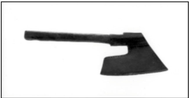
Figure 16—An 18th-century Germanic goose-wing hewing ax. There are maker’s marks hammered into the blade.
