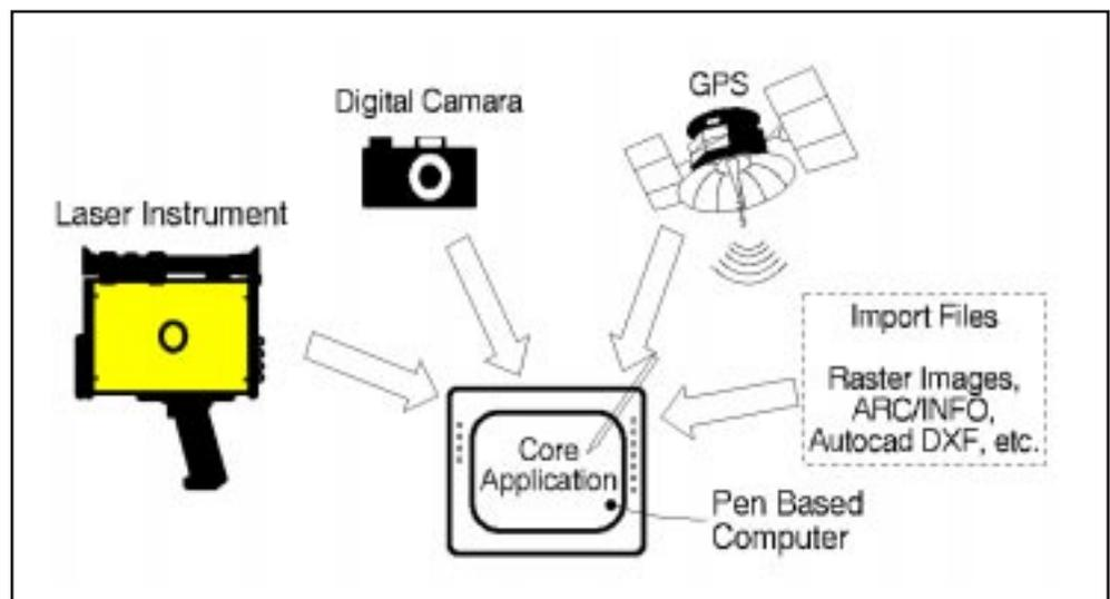
**Figure 1.** Various input devices of a field data collection/mapping system
